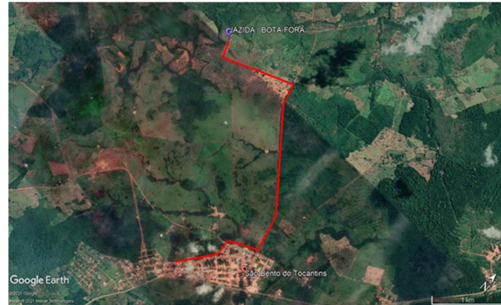
JAZIDA / BOTA-FORA [DMT 1 = 4,0km] [DMT 2 = 7,2km] S/ESCALA
